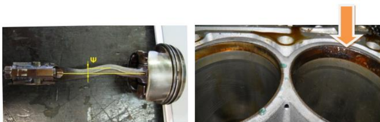
Fig.5. The typical shape of a connecting rod during buckling due to a hydrolock in cylinder [5] fully corresponds to the calculated one (left), and the expansion of the carbon deposits in the upper part of the cylinder (right) when working with a conrod deformed during a hydrolock makes it possible to unambiguously measure its deformation even after destruction
